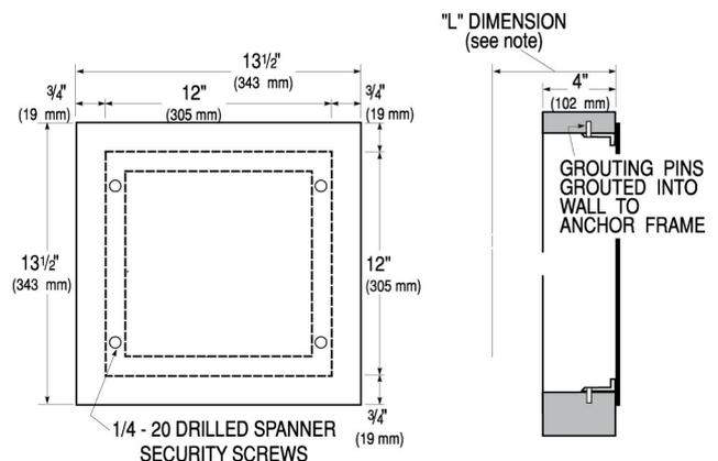
NOTE: "L" Dimension is the Wall Thickness (to the nearest whole inch) plus 2¾". Specify "L" Dimension when ordering Flushometer.
